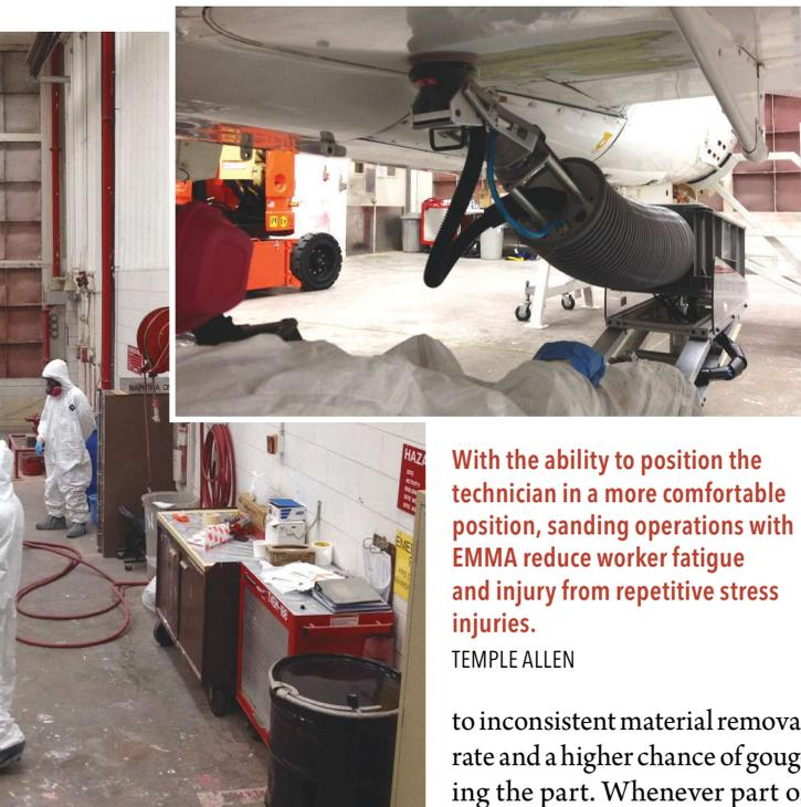
**With the ability to position the technician in a more comfortable position, sanding operations with EMMA reduce worker fatigue and injury from repetitive stress injuries.**
