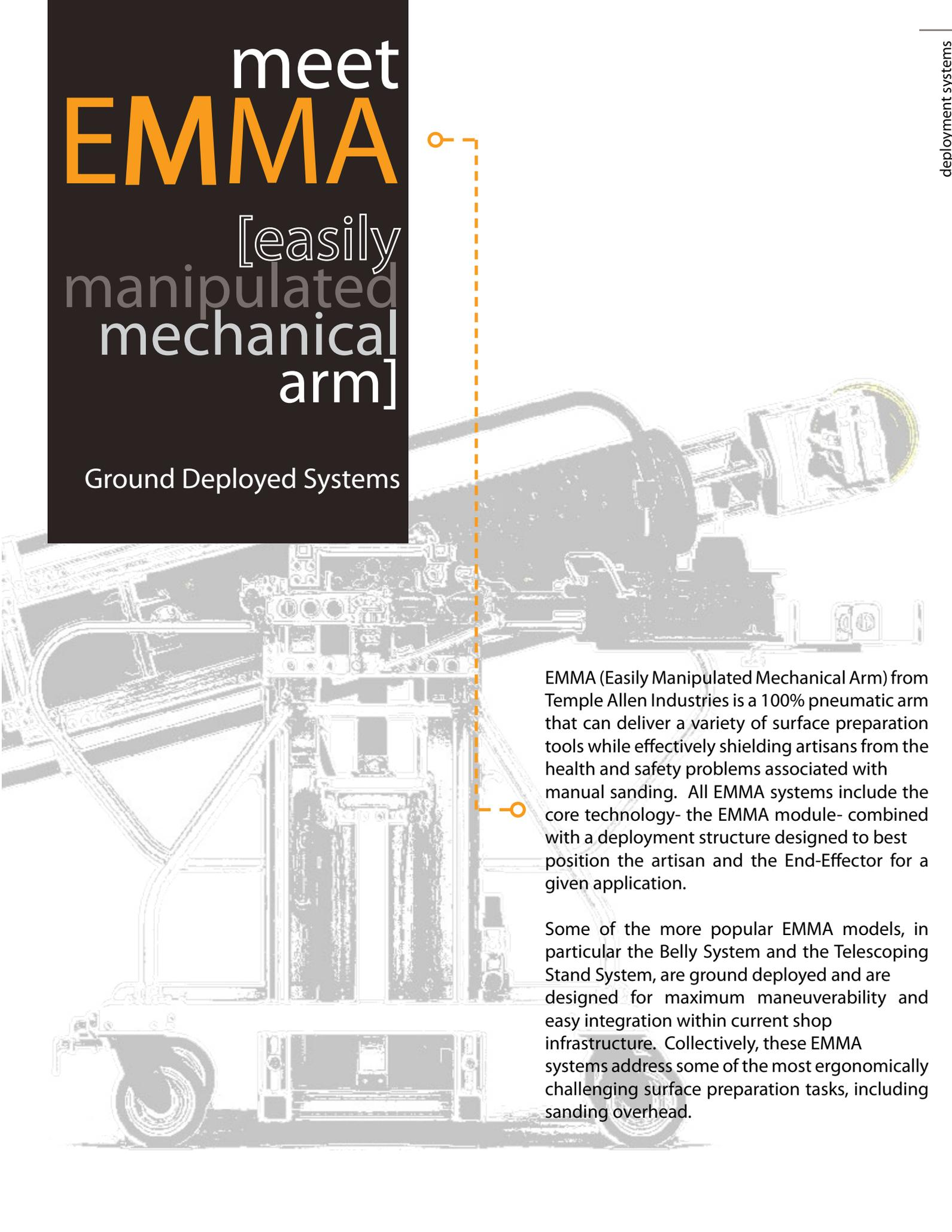
EMMA (Easily Manipulated Mechanical Arm) from Temple Allen Industries is a 100% pneumatic arm that can deliver a variety of surface preparation tools while effectively shielding artisans from the health and safety problems associated with manual sanding. All EMMA systems include the core technology- the EMMA module- combined with a deployment structure designed to best position the artisan and the End-Effector for a given application.
